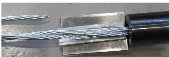
Figure 6. Test object No. 3, location of fracture.
