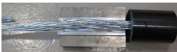
Figure 4. Test object No. 1, location of fracture.
