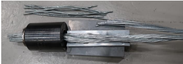
Figure 4. Test object No. 1, location of fracture.
