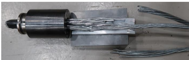
Figure 6. Test object No. 3, location of fracture.
