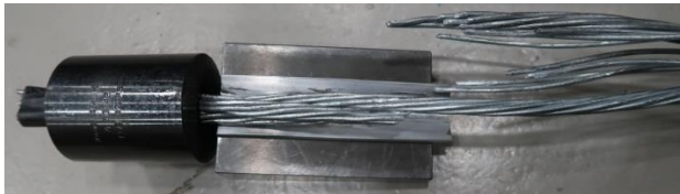
Figure 5. Test object No. 2, location of fracture.
